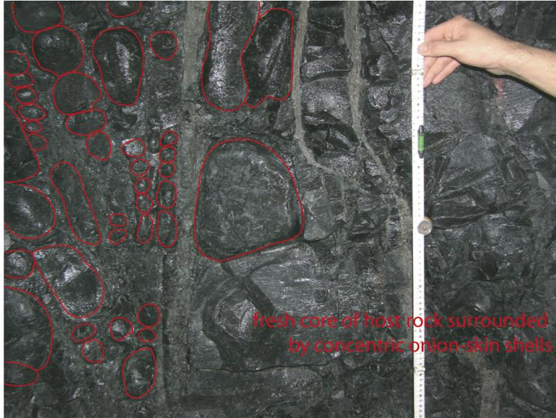
Kimberlite dyke – damage zone + preconditioning
